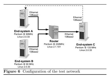
PC with a Pentium CPU running at 200 MHz is sufficient to route incoming traffic of 20 Mbit/s at least.
