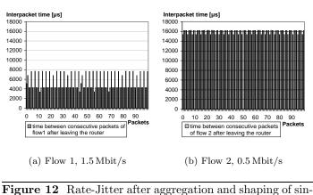
Figure 12 Rate-Jitter after aggregation and shaping of single flows in a border router
